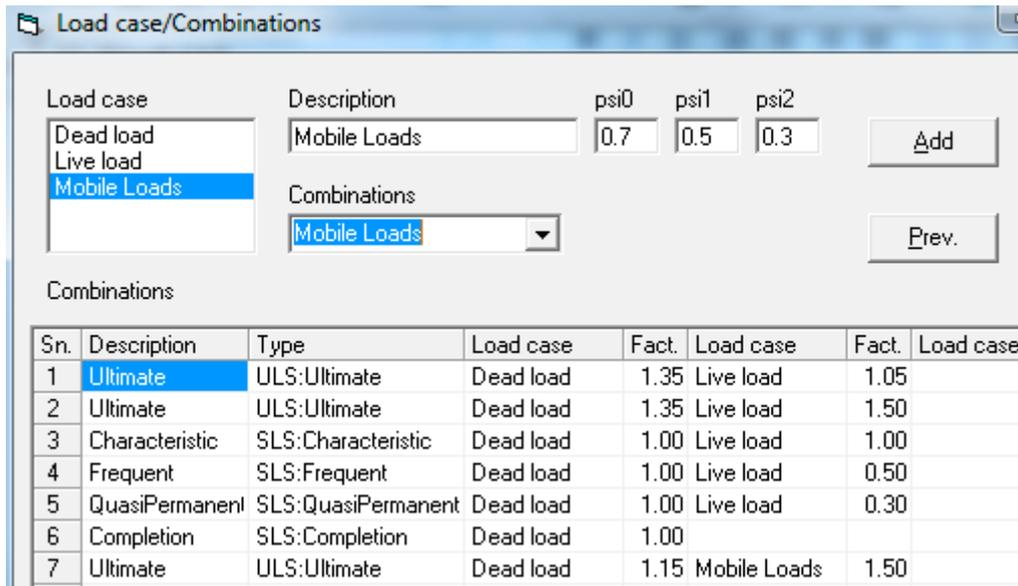
If a mobile loading is entered Tab Mobile Loads is shown. Passing Axle load is an option in the pull down menu and a following axle load. The are moved with a displacement value in the column after the load value. Each passing hindrance to one or more axes are added next. Q- and P-loads are only single state treated.
