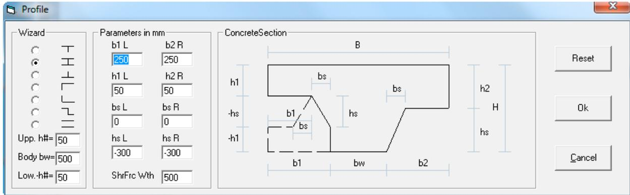
$h1$  Or  $h2$  is chosen then the rebate is at the top. In the calculation, and on paper, the intersection will be compressed at the Y-axis which presents the view slightly different. An H-profile seems impossible but isn't, eg  $H = 300$ ,  $B = 1000$ ,  $h1 = 100$ ,  $b1 = 300$ ,  $h2 = -100$ ,  $b2 = 300$
