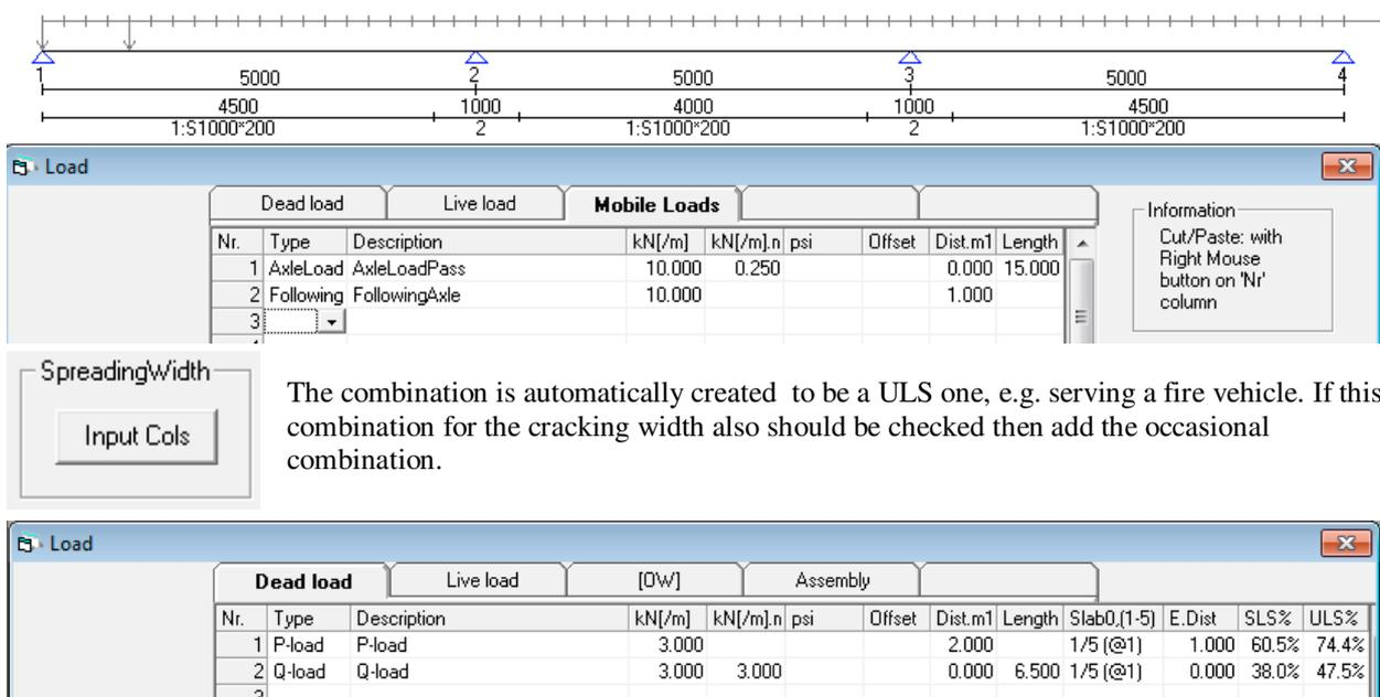
Loads sharing with slab floors is possible under NEN - EN 1168 (Annex C). The button on the left will add 4 columns to do so. The columns relate succ. the edge distance and the calculated plate  $\alpha$  t/m  $\alpha$ 5 for determining V/H share on usability and ultimate limit state . The proportion may be adjusted.
