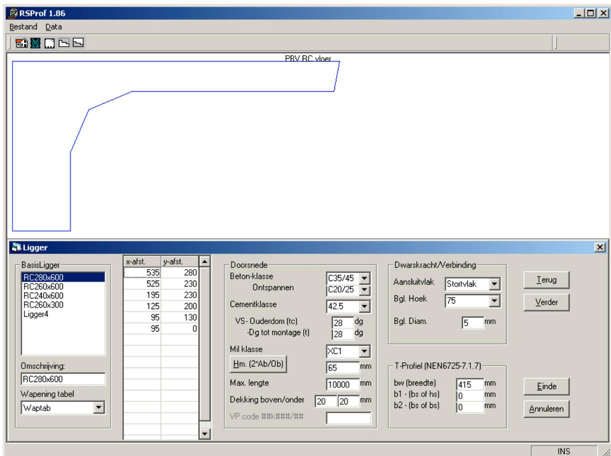
Because only the x-axis is relevant when solving, the cross-section can be compressed on the y-axis.
