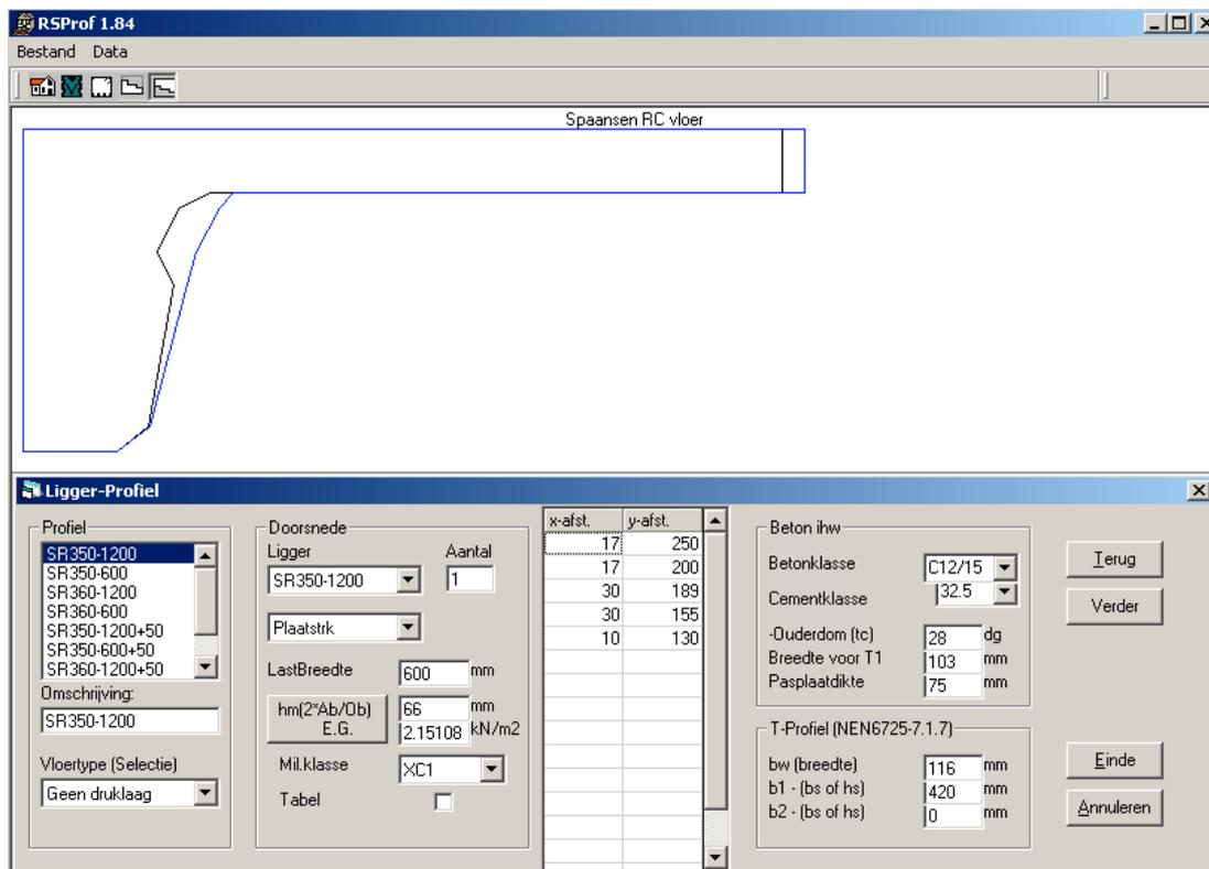
If something is changed that causes the factor  $h_0 = (2A_c/u)$  and OW (may be overruled), to change the amounts the values will be colored red. With the button next to the red values, a recalculation is made and the relevant values are entered in 't black.
