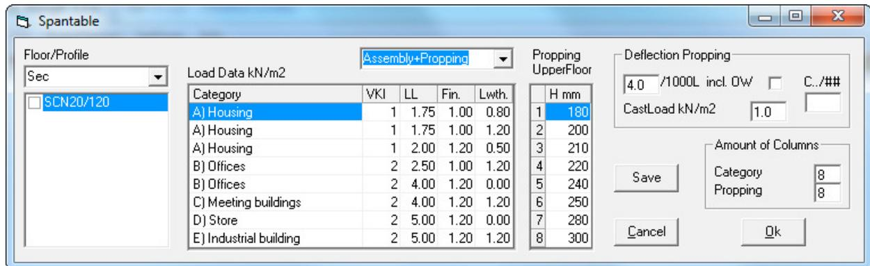
Now floor types with matching profiles are to be selected. The profiles in the table are defined in its profile file that may be customised with RSPProf.exe. Choose the way the table is to be made: with or without mounting support, and with load of an overhead concrete floor while assembling it.
